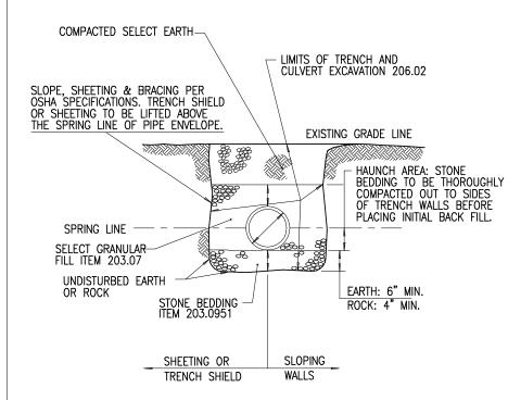
WHERE DRAIN LINE CROSSES PREVIOUSLY INSTALLED SANITARY SEWER, WATER OR GAS MAIN, ETC. TRENCH SHALL BE EXCAVATED DOWN TO THE PREVIOUSLY LAID CONDUIT AND BACKFILLED WITH COMPACTED #2 CRUSHER RUN STONE TO INSURE ADEQUATE SUPPORT.
